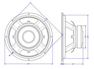
Mounting Details Baffle opening diameter: front mounting 233 mm Mounting pattern: Eight 5.0 mm holes eqi-spaced on a 245mm P.C.D. Flange thickness 8.3mm
